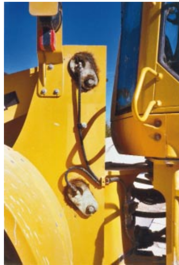
Lubrication lines serve the lift arm cylinder and the lift arm hinge pin of this Caterpillar 980G. The grease seal is visually apparent.
