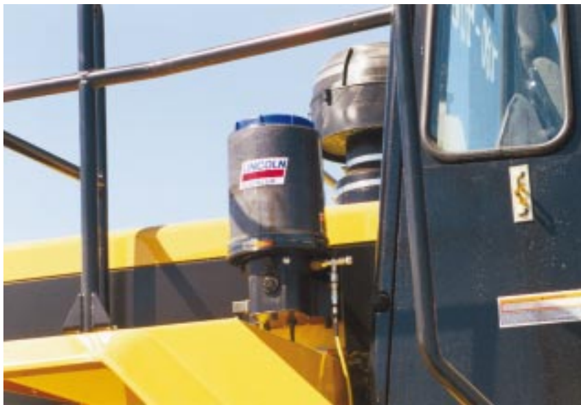
This Caterpillar 980G wheel loader is equipped with a lubrication system powered by a Lincoln Quicklub 203 pump with 8-liter reservoir.
